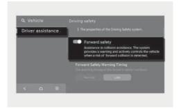
With the vehicle on, select **Settings** > **Vehicle** > **Driver assistance** > **Driving safety** in the infotainment system to set whether to use each function.
