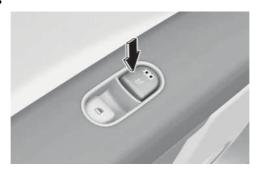
While the vehicle is running, press the seat warmer switch to warm the rear seat.
