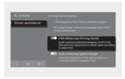
With the vehicle on, select or deselect **Settings** > **Vehicle** > **Driver assistance** > **Driving Convenience** > **HDA (Motorway Driving Assist)** from the infotainment system to set whether to use each function.
