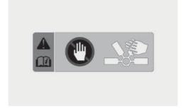
When using the V2L, the cooling fan in the vehicle motor compartment can operate automatically even if the vehicle is turned off. Do not put your hand near the cooling fan in the V2L operating state.
