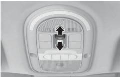
The power sunshade can only be operated when Start/Stop button is in the ON or START position.
