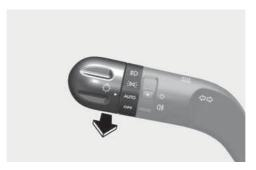
To flash the high beam headlight, pull the lever towards you, then release the lever. The high beams remain ON as long as you hold the lever.
