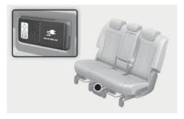
V2L(Vehicle to Load) is installed at the central rear seat bottom. V2L is a convenient feature which provides enough electricity to use diverse household electrical appliances in the vehicle.
