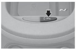
Press the Parking Safety (P<sup>m/2</sup>) button to turn on Forward/Reverse Parking Distance Warning. Press the button again to turn off the function.
