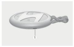
2 Remove the old battery and insert a new battery. Make sure the battery position is correct. An improperly positioned battery may discharge the battery, causing smart key failure.
