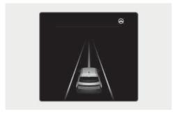
If the vehicle ahead and/or both lane markings are detected and your vehicle speed is below 200 km/h (120 mph), the green (a) indicator light appears on the cluster, and Lane Following Assist helps center the vehicle in the lane by assisting the steering wheel.
