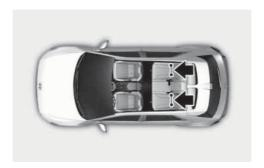
ISOFIX anchorages have been provided in the left and right outboard rear seating positions. Their locations are shown in the illustration. There are no ISOFIX anchorages provided for the center rear seating position.
