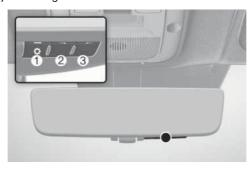
1 Press the menu button (1). You can adjust the brightness and the vertical angle of the display.
