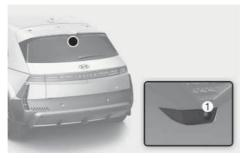
• If the camera lens (1) is dirty, the displayed image may not be clear. In this case, clean it with a soft cloth dampened with water or a swab.
