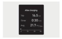
Trip distance, total driving time, average energy consumption, and instant energy consumption after the vehicle has been recharged are displayed. To reset manually, press the **OK** button on the steering wheel for more than 1 second when "After charging" appears.
