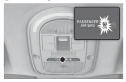
Insert the key or a similar rigid device into the passenger's front airbag ON/OFF switch and turn it to the ON position [A]. The passenger airbag ON indicator (®) illuminates.
