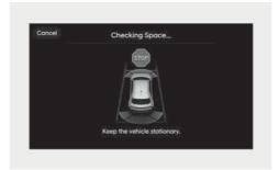
When the vehicle is stopped by depressing the brake pedal, the vehicle sensors will detect the distance from nearby objects and check for space to exit.
