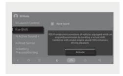
• When N e-Shift is activated, the sound of N Active Sound+ will automatically turn to ignition mode.
