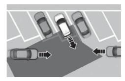
Rear Cross-Traffic Collision-Avoidance Assist may be limited when backing up diagonally, and may not detect the vehicle approaching from the left or right. If this occurs, the function may not warn the driver or control the brakes when necessary. Always check your surroundings while backing up.
