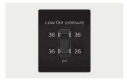
When the tire pressure monitoring system warning indicator ((1)) is illuminated and a warning message appears on the cluster display, one or more of your tires is significantly under-inflated. The Low Tire Pressure Position Telltale will indicate which tire is significantly under inflated by illuminating the corresponding position light.
