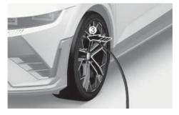
12 Plug the compressor power cord into the vehicle power outlet.
