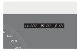
The main settings of CUSTOM mode is displayed at the top of the cluster. The CUSTOM mode can be set on the infotainment system.
