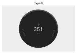
The distance to empty is the estimated distance the vehicle can be driven with the remaining electric energy.
