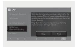
Depending on the current and target temperature, heater/chiller will be adjusted and the estimated time will be displayed accordingly.
