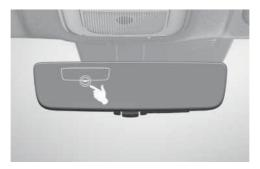
If the symbol shown in the illustration is displayed when using the Digital Center Mirror in digital mirror mode, the system may be malfunctioning. The symbol will disappear in a few seconds. Operate the lever, change to optical mirror mode and we recommend that you have the vehicle inspected by an authorized HYUNDAI dealer.
