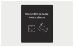
When Highway Driving Assist is operating, your vehicle will stop if the vehicle ahead of you stops. Also, if the vehicle ahead of you starts moving within 30 seconds after the stop, your vehicle will start as well. In addition, after the vehicle has stopped and 30 seconds have passed, the "Use switch or pedal to accelerate" message will appear on the instrument cluster. Depress the accelerator pedal or operate the + switch, - switch or IIIO switch to start driving.
