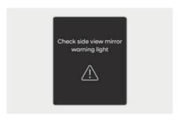
When the outside rearview warning light is not working properly, the "Check side view mirror warning light" (or "Check outside mirror warning icon") warning message will appear on the instrument cluster for several seconds, and the master (A) warning light will illuminate on the instrument cluster. If this occurs, we recommend that your vehicle be inspected by an authorized HYUNDAI dealer.
