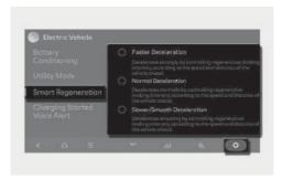
To adjust the regenerative braking level of the smart regeneration system, select **Electric Vehicle** > ★ > Smart Regeneration in the infotainment system.
