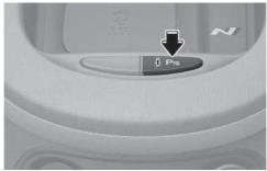
Press and hold the Parking Safety ( $P_{i,k}$ ) button more than 2 seconds, 'Rear Active Assist' or to turn the Parking Collision-Avoidance Assist on or off.
