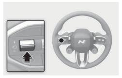
Press the II a switch to temporarily pause the set speed limit. The set speed limit will turn off but the Speed Limit (O'LIMIT) indicator will stay on.
