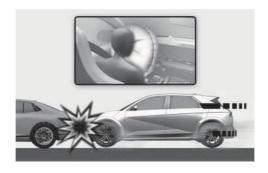
Front airbags are designed to inflate in a frontal collision depending on the severity of impact.
