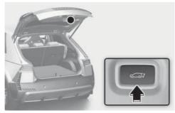
Press the power tailgate open/close button. The tailgate opens or closes automatically.
