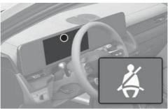
As a reminder to the driver, the driver's seat belt warning lights illuminates for about 6 seconds each time the Start/Stop button is in the ON position regardless of seatbelt fastening.
