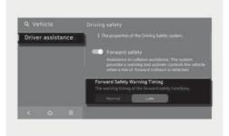
With the vehicle on, select Settings > Vehicle > Driver assistance > Driving safety > Forward Safety Warning Timing in the infotainment system to change the initial warning activation time for Forward Collision-Avoidance Assist. The warning time can be set to either "Normal" or "Late"
