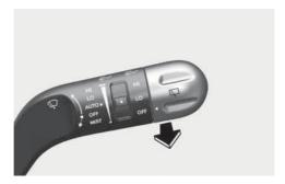
In the OFF(O) position, pull the lever gently toward you to spray washer fluid on the windshield and to run the wipers 1-3 cycles. The spray and wiper operation continues until you release the lever. If the washer does not work, you may need to add washer fluid to the washer fluid reservoir.
