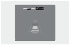
If you want to speed up temporarily without altering the set speed while Smart Cruise Control is operating, depress the accelerator pedal. While the accelerator pedal is depressed, the set speed, distance level and target distance will blink on the cluster. However, if the accelerator pedal is depressed insufficiently, the vehicle may decelerate.
