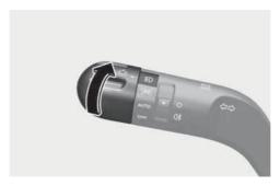
The headlight, position light, license plate light and instrument panel lamp are turned ON.
