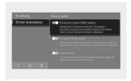
With the vehicle on, select **Settings > Vehicle > Driver assistance > Driving safety > Forward cross-traffic safety** in the infotainment system to turn on Junction Crossing function and deselect to turn off the function.
