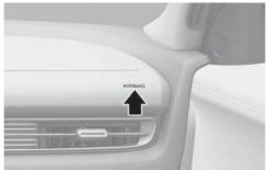
The SRS consists of airbags located in the center of the steering wheel and the passenger's side front panel pad above the glove box.
