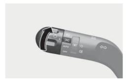
The position light, license plate light, and instrument panel lamp are turned ON.
