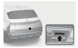
When the tailgate is closed, press the power tailgate open/close button to open the tailgate.
