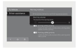
With the vehicle on, go to **Settings** > **Vehicle** > **Driver assistance** > **Warning methods** from the Settings in the infotainment system to select the following:
