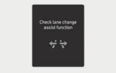
When Highway Driving Assist is not working properly, the "Check driver assistance system." and "Check lane change assist function" warning message and the master (A) warning light appears on the instrument cluster. If this occurs, we recommend that your vehicle be inspected by an authorized HYUNDAI dealer.
