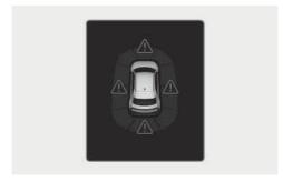
When the Parking Distance Warning is operating, if the function is not working normally or the ultrasonic sensor is blocked, the master warning light (<u>A</u>) appears in the direction of the corresponding sensor. You can check the warning in the Utility view on the cluster.
