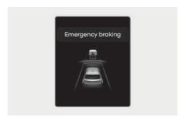
To warn the driver that emergency braking will be assisted, the "Emergency braking" warning message will appear on the cluster, an audible warning will sound.
