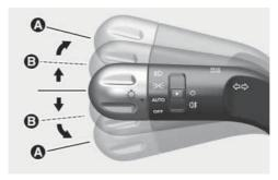
To signal a turn, push down on the lever for a left turn or up for a right turn in position [A]. If an indicator stays on and does not flash or if it flashes abnormally, one of the turn signal bulbs may be burned out and may require replacement. We recommend that you contact an authorized HYUNDAI dealer.
