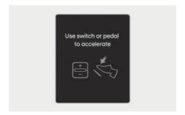
In traffic, your vehicle will stop if the vehicle ahead of you stops. Also, if the vehicle ahead of you starts moving, your vehicle will start as well. In addition, after the vehicle has stopped and a certain time have passed, the "Use switch or pedal to accelerate" message will appear on the instrument cluster. Depress the accelerator pedal or operate the + switch. - switch or II > switch to start driving.
