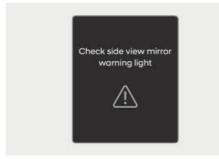
When the side view mirror warning light is not working properly, the "Check side view mirror warning light" (or "Check outside mirror warning icon") warning message will appear on the instrument cluster for several seconds, and the master (小) warning light will appear on the instrument cluster. If this occurs, we recommend that your vehicle be inspected by an authorized HYUNDAI dealer.
