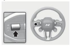
Press the | Switch or depress the brake pedal to temporarily cancel Smart Cruise Control.
