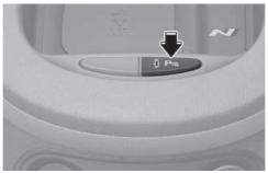
Press and hold the Parking Safety ( $P_{\text{NL}}$ ) button more than 2 seconds, to turn the Parking Collision-Avoidance Assist on or off.
