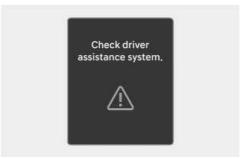
When Safe Exit Warning is not working properly, the "Check driver assistance system." warning message will appear on the cluster for several seconds, and the master warning light (A) will appear on the cluster. If this occurs, we recommend that your vehicle be inspected by an authorized HYUNDAI dealer.
