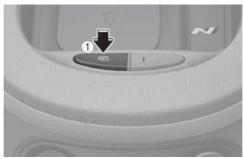
Press the Parking/View button (1) to turn on Surround View Monitor. Press the button again to turn off the function.
