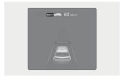
When Based on Driving Style is operating, the vehicle distance level and target distance will be displayed white based on the driving style.
