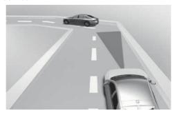
The front sensors may be unable to recognize the foregoing vehicle if you are coasting on a curve. The regenerative braking intensity may automatically be lowered, which may accelerate the vehicle.
