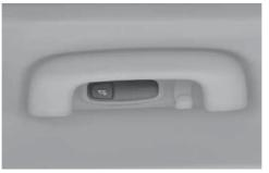
$\nabla$ ,  $\nabla$ : Press the button to turn on and off the rear room lamp.
