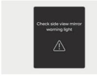
When the side view mirror warning light is not working properly, the "Check side view mirror warning light" (or "Check outside mirror warning icon") warning message appears on the instrument cluster for several seconds, and the master (A) warning light illuminates on the cluster. If this occur, we recommend that your vehicle be inspected by an authorized HYUNDAI dealer.
