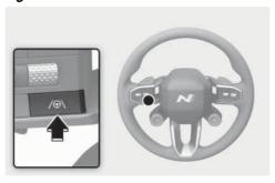
With the vehicle on, shortly press the Lane Driving Assist button located on the steering wheel to turn on Lane Following Assist. The gray or green (A) indicator light will appear on the cluster.
