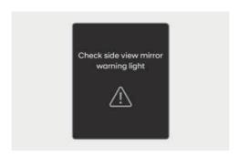
When the side view mirror warning light is not working properly, the "Check side view mirror warning light" (or "Check outside mirror warning icon") warning message will appear on the cluster for several seconds, and the master warning light (A) will appear on the cluster. If this occurs, we recommend that your vehicle be inspected by an authorized HYUNDAI dealer.
