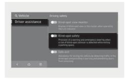
With the vehicle on, select **Settings > Vehicle > Driver assistance > Driving safety > Blind-spot safety** in the infotainment system to set whether to use each function.
