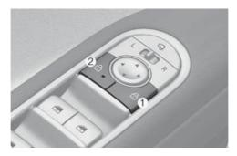
When pressing the  $\bigcirc$  portion (1) on the switch, all vehicle doors are locked.
