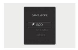
The mode changes, whenever the N1 or N2 button on the steering wheel or the Drive mode button is pressed.
