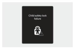
When electronic child safety lock does not work even though the button is pressed, the message will be displayed and an alarm will sound. If this occurs, we recommend that the vehicle be inspected by an authorized HYUNDAI dealer.
