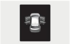
This warning appears if any door or hood or tailgate is left open. The warning indicates which door is open on the cluster display.
