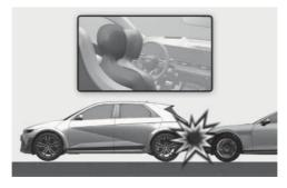
Front airbags are not designed to inflate in rear collisions, because occupants are moved backward by the force of the impact.
