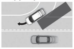
Blind-Spot Collision-Avoidance Assist may not operate properly when driving where the road merges or divides. The function may not detect the vehicle in the next lane. Always pay attention to road and driving conditions while driving.
