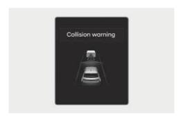
While Smart Cruise Control is operating, when the collision risk with the vehicle ahead is high, the "Collision Warning" warning message will appear on the instrument cluster, and an audible warning will sound to warn the driver. Always have your eyes on the road while driving, and if necessary, depress the brake pedal to reduce your driving speed in order to maintain a safe distance.
