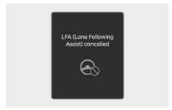
If the driver still does not have their hands on the steering wheel after the hands-off warning, the "LFA (Lane Following Assist) cancelled" (or "Lane Following Assist deactivated") warning message will appear and Lane Following Assist will be automatically cancelled.
