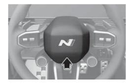
To sound the horn, press the area indicated by the horn symbol on your steering wheel (see illustration). The horn operates only when this area is pressed.
