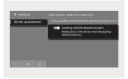
With the vehicle on, select or deselect **Settings** > **Vehicle** > **Driver assistance** > **DAW** (**Driver Attention Warning**) and then enable **Leading vehicle departure alert** in the infotainment system to set whether to use each function.
