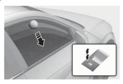
If a window senses any obstacle while it is closing automatically, it stops and lowers about 30 cm (12 in.) to allow the object to be cleared.
