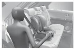
If your Child Restraint System manufacturer instructs or recommends you to use a top tether anchorage with the lap/shoulder belt, refer to "Securing a Child Restraint System seat with Top Tether Anchorage system" section for more information.
