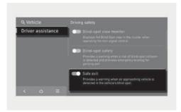
With the vehicle on, select Settings > Driver assistance > Driving safety > Safe exit in the infotainment system to turn on Safe Exit Warning and deselect to turn off the function.
