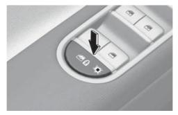
When the electronic child safety lock (1) button is in the LOCK position and an approaching vehicle from the rear area is detected, the electronic child safety lock button will not unlock even if the driver presses the button to prevent the rear doors from opening.
