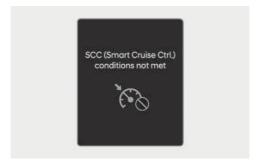
If the Driving Assist button, + switch, - switch or II > switch is operated when Smart Cruise Control operating conditions are not satisfied, the "SCC (Smart Cruise Ctrl.) conditions not met" (or "Smart Cruise Control conditions not met") will appear on the cluster, and an audible warning will sound.
