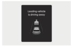
When a detected vehicle in front departs from a stop, Leading Vehicle Departure Alert will inform the driver by displaying the "Leading vehicle is driving away" (or "Leading vehicle is driving on") message on the instrument cluster and an audible warning will sound.
