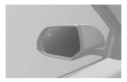
Your vehicle is equipped with both left-hand and right-hand side view mirrors. The mirrors can be adjusted with the mirror adjustment control switch. Adjust the rearview mirrors to your desired position before driving. The side view mirrors can be folded to help prevent damage when going through an automatic car wash or when passing through a narrow street.
