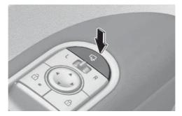
The side view mirrors can be folded or unfolded by pressing the button.
