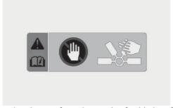
Keep hands, clothing, and tools away from the rotating fan blades of the cooling fan. The electric motor for the cooling fan may continue to operate or start up when the vehicle is off and can cause serious injury.
