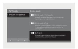
With the vehicle on, select Settings > Driver assistance > Driving safety > Safe exit from the Settings menu to turn on Safe Exit Assist and deselect to turn off the function.
