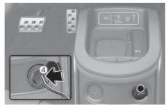
6 With the vehicle ON (READY indicator ON), switch on the compressor and let it run for about 5-7 minutes to fill the sealant up to proper pressure. (refer to the "Tires
