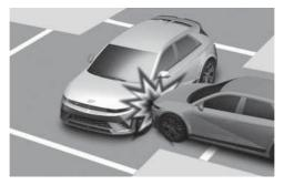
Front airbags may not inflate in side impact collisions, because occupants move in the direction of the collision.
