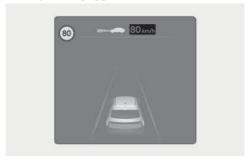
Manual Speed Limit Assist or Smart Cruise Control assists the vehicle to adjust its speed according to the speed limit. When the cruising speed is set as same as the speed limit, the vehicle automatically adjusts its speed if the speed limit changes. The function operates on the road which has a speed limit of 70 km/h (45 mph) or higher. When the function is active, the cruising speed on the instrument cluster appears in green.
