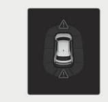
When the Parking Distance Warning is operating, if the function is not working normally or the ultrasonic sensor is blocked, the master warning light (<u>A</u>) appears in the direction of the corresponding sensor. You can check the warning in the Utility view on the cluster.
