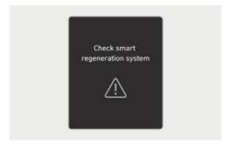
If the smart regeneration system is turned off due to the front radar being covered with foreign substances or due to other causes, the "Check smart regeneration system" warning message appears. Also the regenerative braking level is displayed instead of 'AUTO'.
