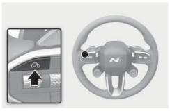
Press the Driving Assist (A) button to turn Manual Speed Limit Assist off. The Speed Limit (білыт) indicator will go off.
