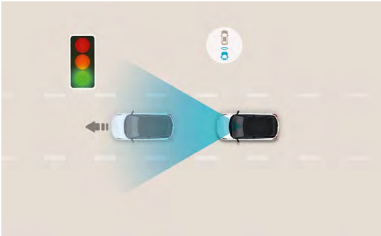
Leading Vehicle Departure Alert (LVDA) .
