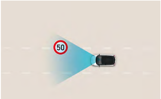
Intelligent Speed Limit Assist (ISLA) .
