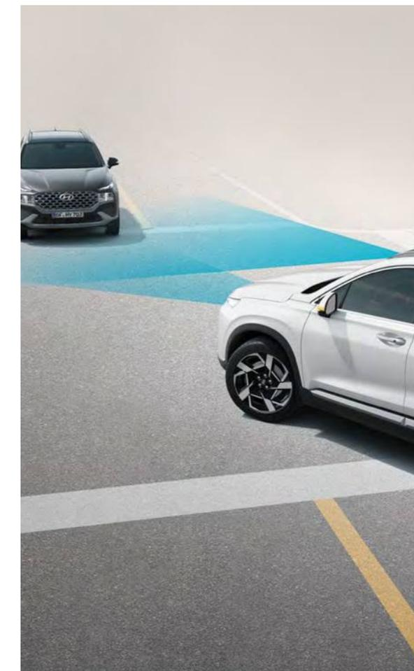
**Forward Collision Avoidance Assist (FCA, Junction Turning)**
