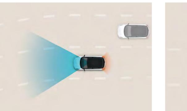
**Navigation-based Smart Cruise Control - Curve (NSCC-C)**
